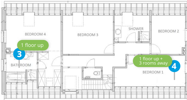
Image: The Excentis Wi-Fi House floor plan with specific points where reproducible readings are taken.
